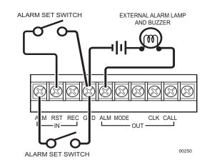
Figure 3. Alarm Recording Connection
